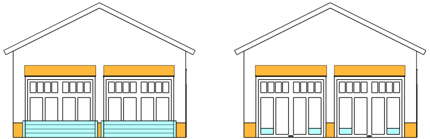
floodproofing examples - screens vs openings
