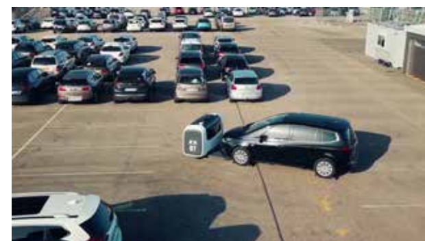
FIG. 4.1.11 AUTOMATED, SELF-VALET © Stanley Robotics
