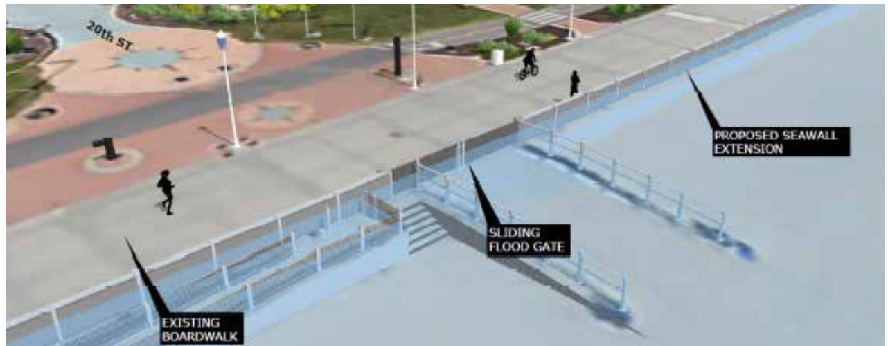
FIG. 4.2.26 RENDERING OF RAISED SEAWALL AND SLIDING FLOOD GATE AT OCEANFRONT BOARDWALK Virginia Beach, Virginia
